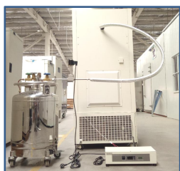
LN 2 /CO 2 backup system
