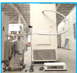
LN 2 /CO 2 backup system
