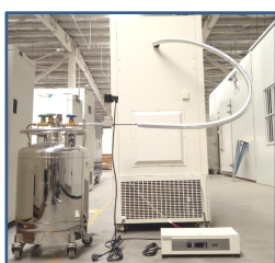
LN 2 /CO 2 backup system
